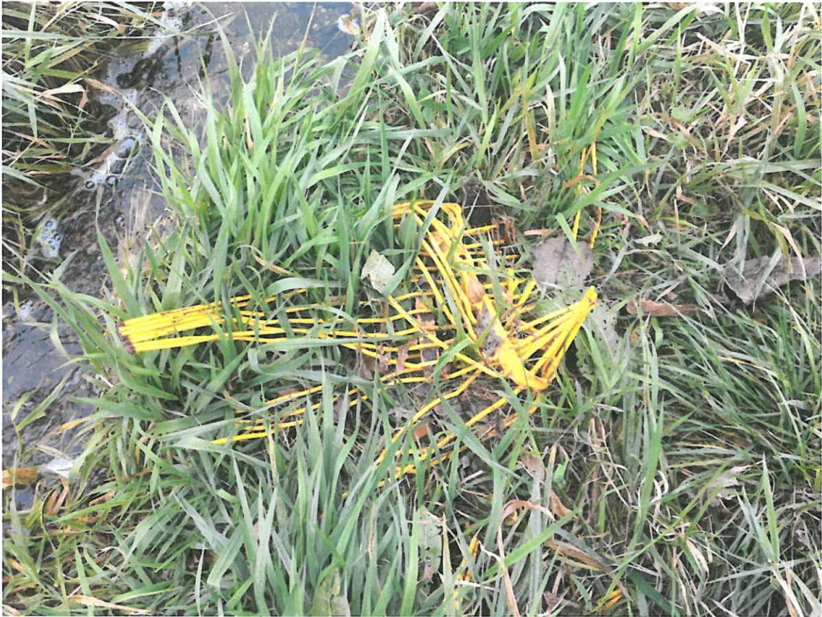
The trash guard completely wrecked. Found in the ditch on the north side of Collins near the water intake.
