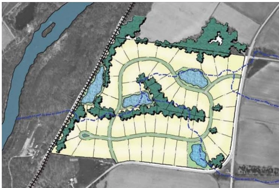
Step 1: Developing a "yield plan" to determine the maximum allowable density for the site.
