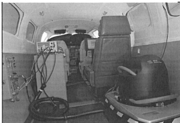
Leica ADS100 installation in a Surdex Cessna 441 (Conquest)
