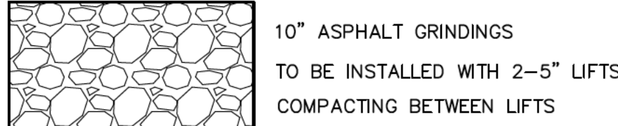
TYPICAL GRAVEL PAVEMENT DETAIL
