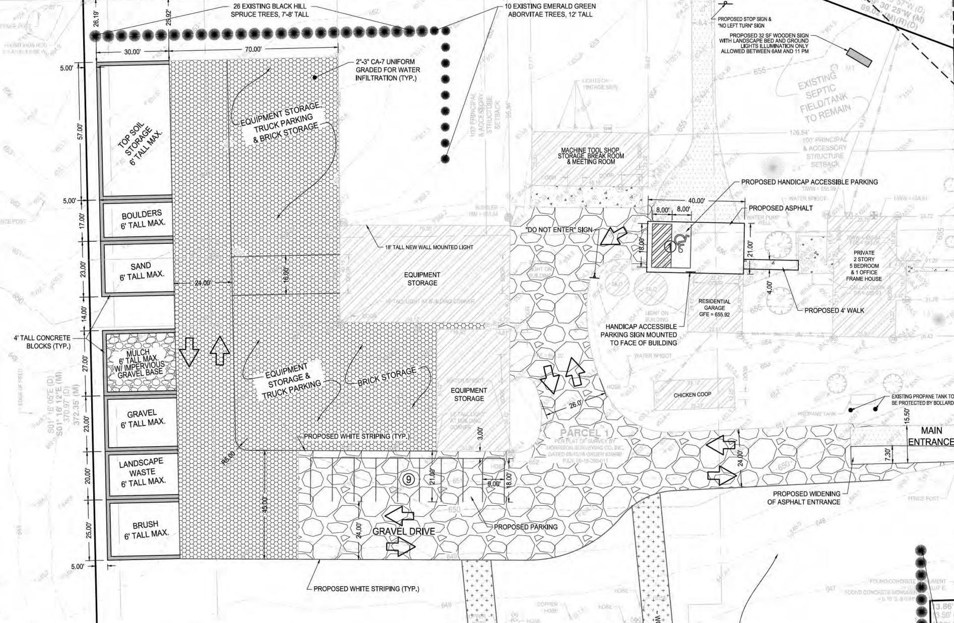
SITE BENCHMARK: CUT CROSS ON THE NORTHEAST CORNER OF THE RIM OF A SQUARE CATCH BASIN LOCATED ON THE WEST SIDE OF GROVE ROAD APPROXIMATELY 11.5 FEET NORTH OF THE DRIVEWAY APRON (CONNECTED TO GROVE ROAD) OF THE SUBJECT PROPERTY. SEE DRAWING FOR EXACT LOCATION. ELEVATION = 650.64 (NAVD 88)
