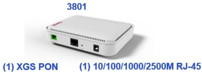
The 3801 provides XGSPON termination to Ethernet at the residence and is capable of speeds from 10Mbps to 2.5Gbps meeting the 100Mbps requirement and exceeding it.
